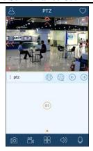
Please control the PTZ by siding the image in direction of the arrow marked on the image. The PTZ will automatically focus on the little red circle by clicking the image. Then the 3D function can be enabled ( the added device must be support 3D function, or this function is ineffective).
